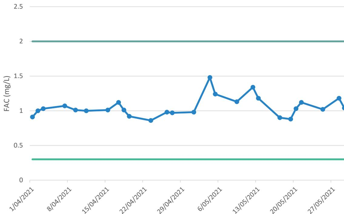
Figure 22: Residual Chlorine of Treated Water from Dargaville WTP
