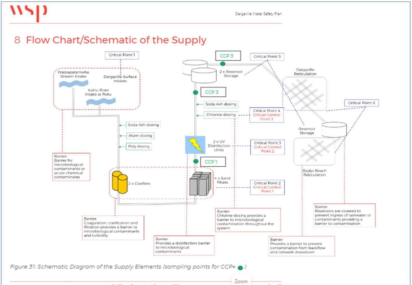
Figure 31: Schematic Diagram of the Supply Elements (sampling points for CCP= ● )
