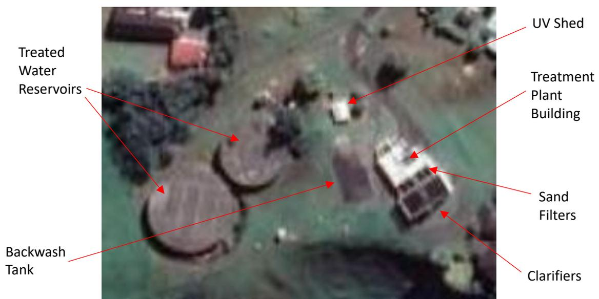
Figure 2: Close up of Dargaville Water Treatment Plant
